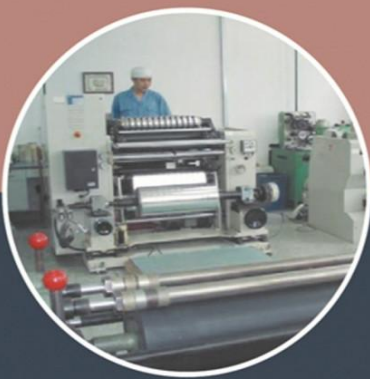
电容器滤波器薄膜分切工序 (引进日本分切设备) Thin film cutting process of capacitors (imported Japanese cutting equipments)
