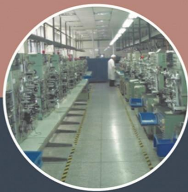
电容器/滤波器芯组卷绕工序 (引进意大利 ARCO牌卷绕机以及日本、韩国、台湾等国 家地区的卷绕机) Winding process of the capacitor core groups (imported Italian ARCO winding machines and other coiling machines from Japan, Korea, Taiwan and other countries and regions)
