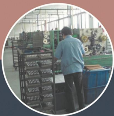
电容器芯组焊接工序（引进日本设备） Welding procedure of capacitor core groups (imported Japanese equipment)
