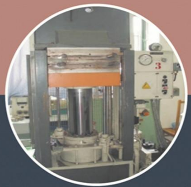
电容器/滤波器芯组热压工序 (引进意大利 2 A 设备) Hot-pressing process of capacitor core groups (imported 2A equipments from Italy)
